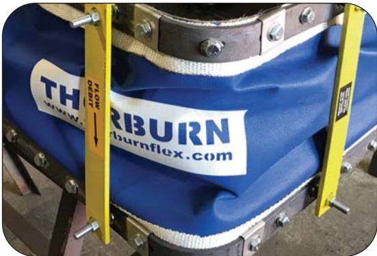
Thorburn's high temperature gaskets are tightly wrapped around the GSM and underneath and beyond the backing bars to reduce leakage and provide protection against heat and abrasion
