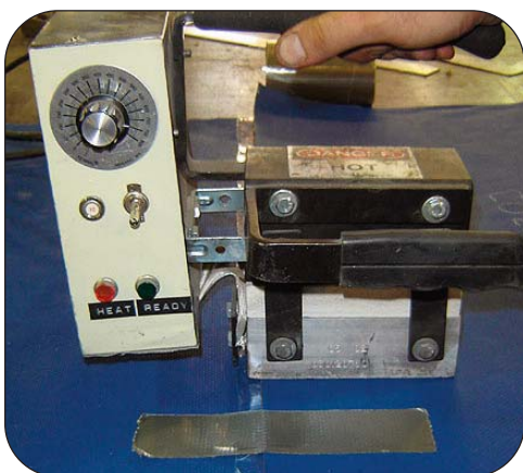
Heating iron in operation on PFA splicing film
