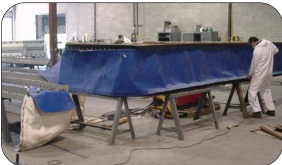
Thorburn Canada technician installing a KLF GSM on a Flexi-Duct™ sectioned outlet expansion joint for an HRSG in Huntstown, Ireland
