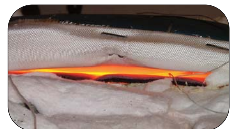
ASTM C-411 Thermal Testing of Thorburn's KLFC GSM with no added insulation to 1100°C
