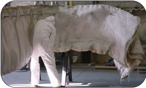
Thorburn's TC-2000RB retaining bag with insulation build-up
