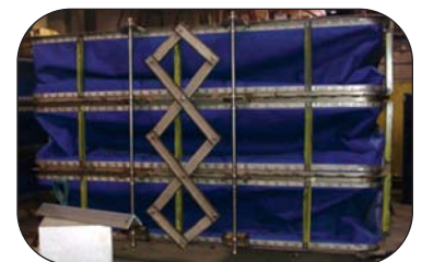
Thorburn's Flexi-Duct™ tertiary expansion joint with a pantograph support system to eliminate hotspot and absorb 600mm (24") lateral and 50mm (2") axial deflection
