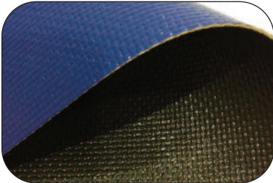
Thorburn's K12 with Thor-Coat 1200 and 2 layers of TLFP
