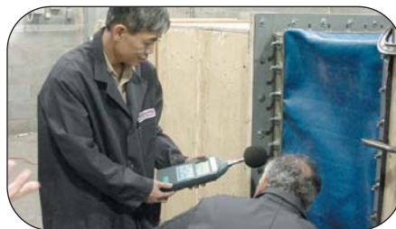
ASTM E596 Acoustic Impedance Testing of Thorburn's Flexi-Duct™ HRSG inlet expansion joint
