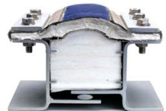
Thorburn's Channel frame with integral liner, pinned cavity pillow with retaining bag and fly ash barrier system
