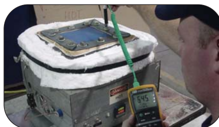
ASTM C411 Cold face GSM and bolt thermal testing of Thorburn's KLF GSM without added insulation
